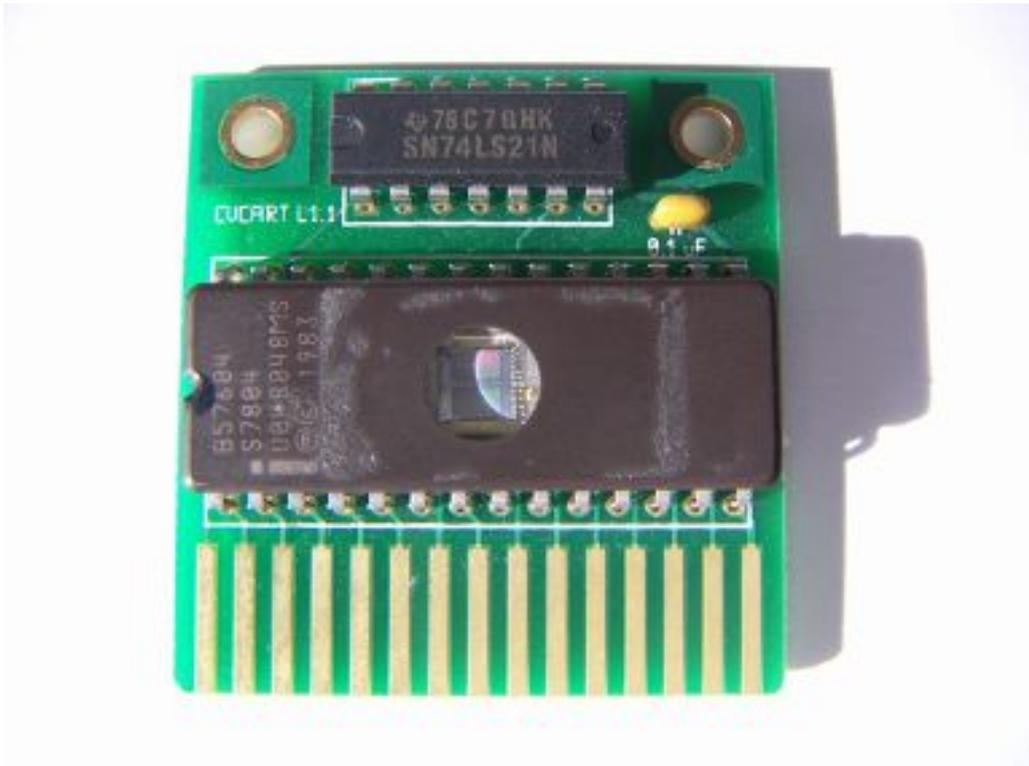
Figure 3: Incorrectly aligned EPROM
