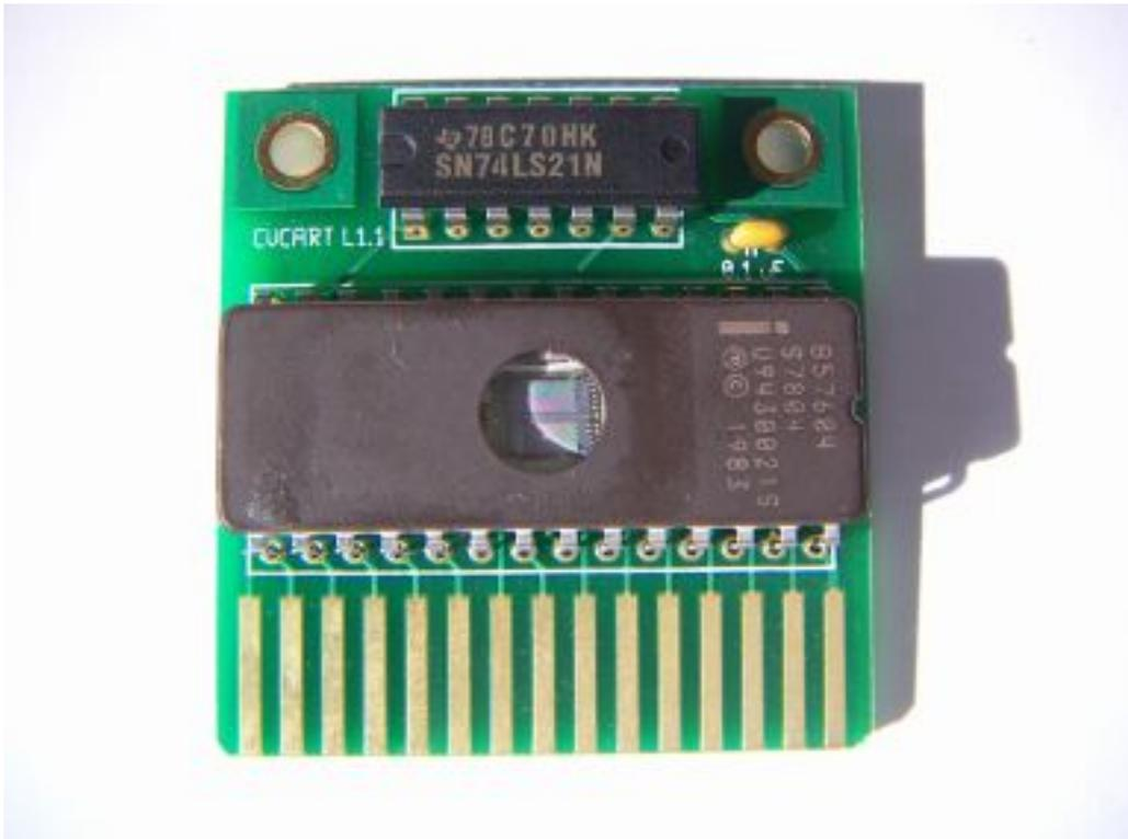
Figure 2: Correctly aligned EPROM and logic chip
